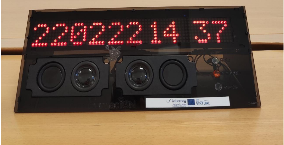
Figure 7 Desktop device. Third version. Text, lights and sound. Hardware upgraded.
