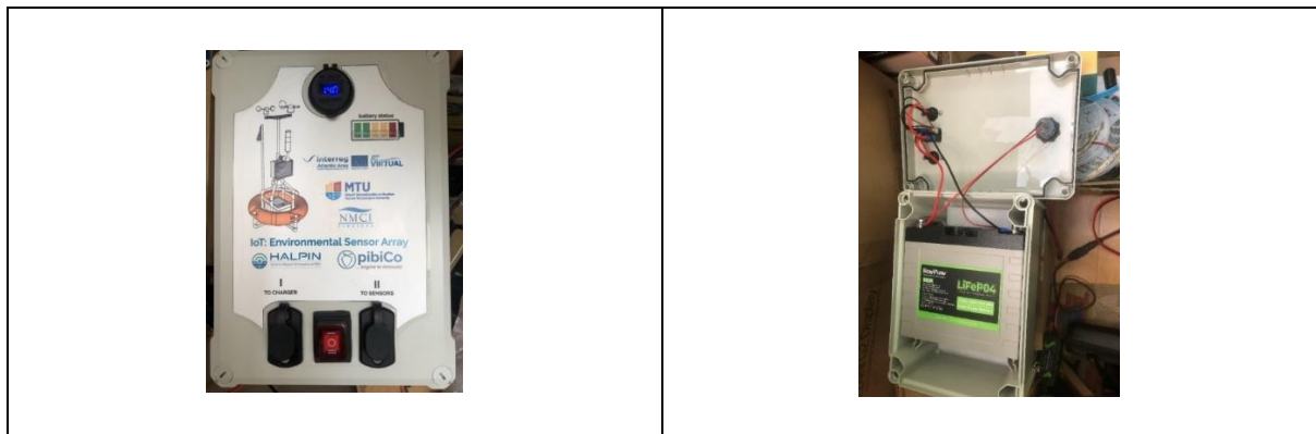
Battery compartment showing waterproof voltage monitor, power switch, connector ports and 18 Ah battery.
